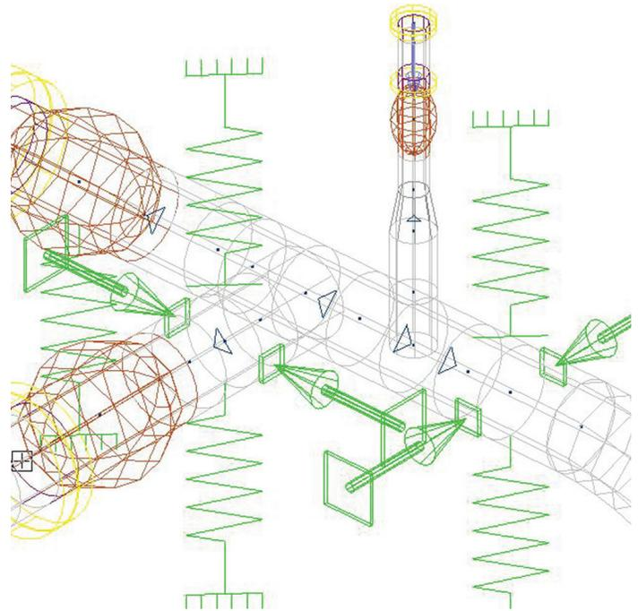
**Figure 2: Blowdown reaction force application.**
