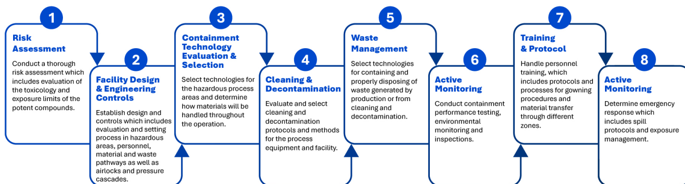
Figure 1: Containment Road map. Steps for managing containment in the pharmaceutical manufacturing process for facilities handling toxic products.
