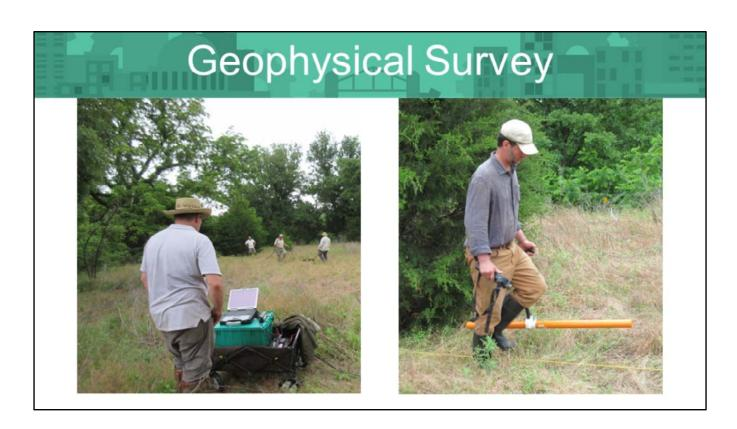
A geophysical survey can be any systematic collection of geophysical data of spatial studies and mapping. Data that is collected using geophysical instruments can be used for mapping subsurface archaeological feature.
