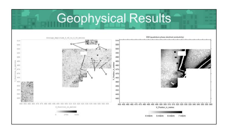
Here are the results for the same location of the site where a geophysical survey took place. The image on the left is the result of the magnetometer survey and the results on the right are from the electromagnetic conductivity survey. Both surveys pinpointed locations where excavations should take place due to the appearance of subsurface features.
